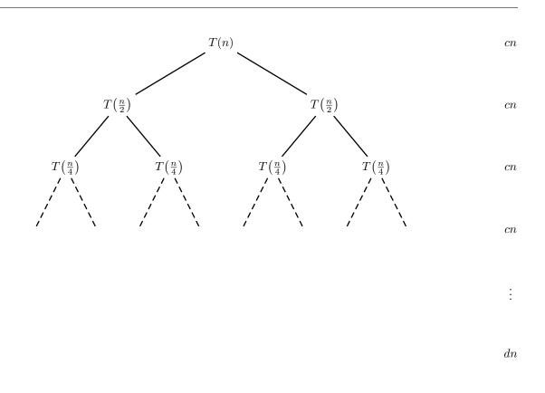
Figure 3: Recursion tree for MERGE-SORT in the simplest case where n is a power of 2.
