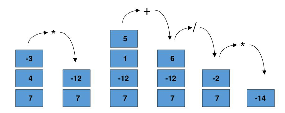
Core of evaluation algorithm using a stack
