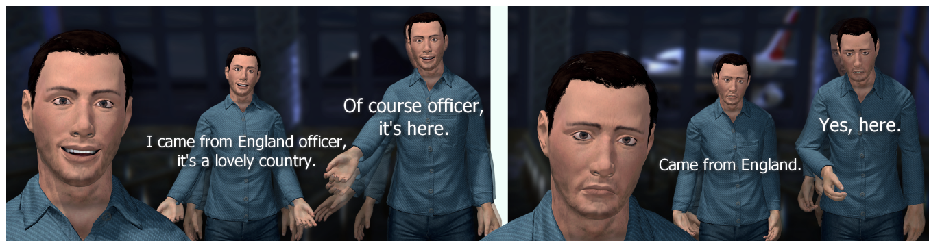
Fig. 1. We adjust voice, body movement, and facial expressions to simulate personalities of virtual agents. The left half shows an extraverted agent, and the right half shows an introverted agent in a scenario involving interaction with a passport officer where the agent responds to questions about his passport and origin. The portraits show the corresponding facial expressions.
