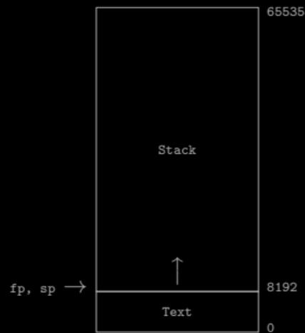
A Marvin program (ie, a `.marv` file) is assembled and loaded into the text segment starting at address 0
