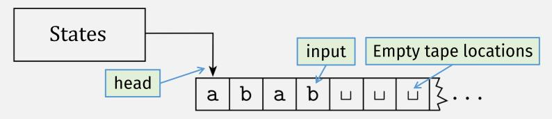
• On a transition, "head" can move left or right 1 step
