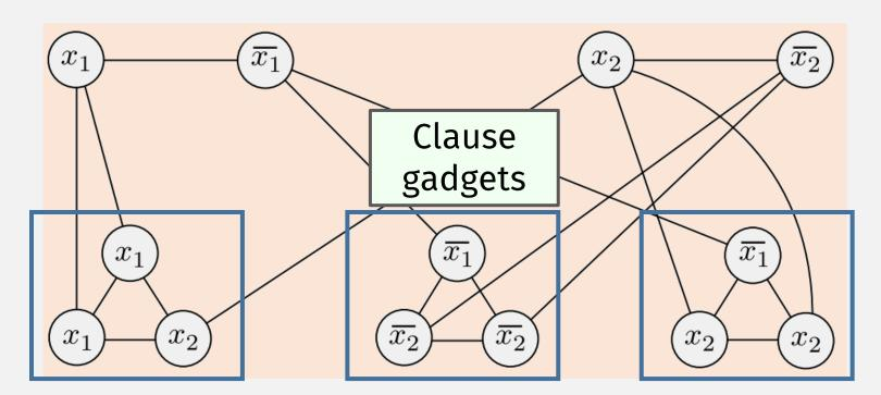
$VERTEX-COVER = \{\langle G, k \rangle | G \text{ is an undirected graph that }$ has a k-node vertex cover $\}$
